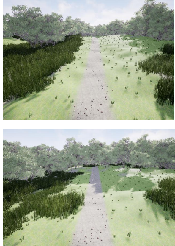
Figure 12: Top: a view in the 3D scene generated from the Adjusted 3 DEM and the original tree and tall grass mask images. Bottom: view from the same vantage point with the same DEM but adjusted tree and tall grass mask images causing different foliage arrangements and densities.
