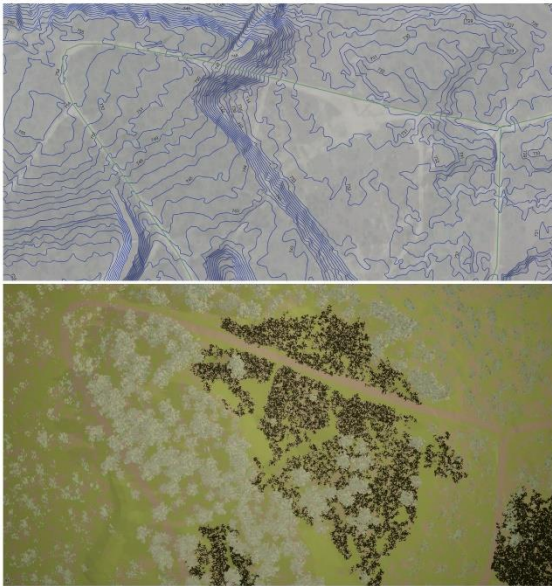
Figure 2: Top: a multi-layer GIS map of a portion of the SwRI Off-Road Test Facility assembled in QGIS. Bottom: an overhead view of the matching portion of the completed 3D scene in UE4.
