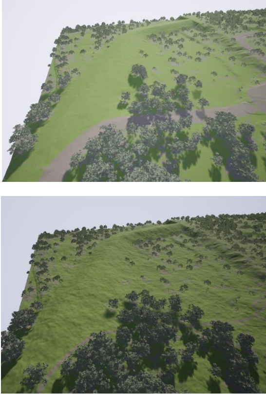
Figure 11: Top: a view of a berm in the SwRI Off-Road Test Facility with the original DEM. Bottom: a similar view with the Adjusted 3 version of the DEM, showing an increased surface roughness.
